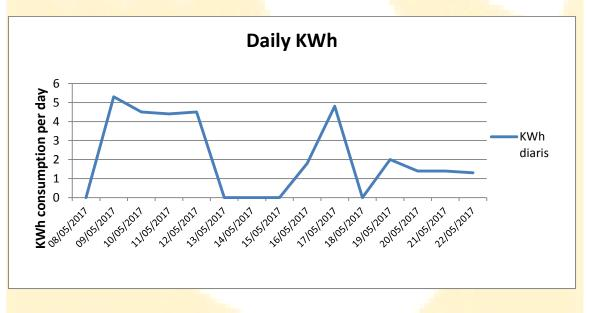
Graphic 6: Daily electric consumption during test 1 and test 2.
