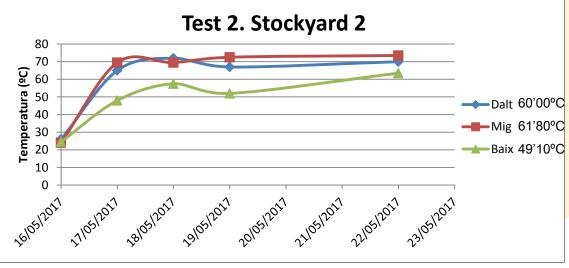
Graphic 4: Temperature curve from Stockyard 2. Test 2
